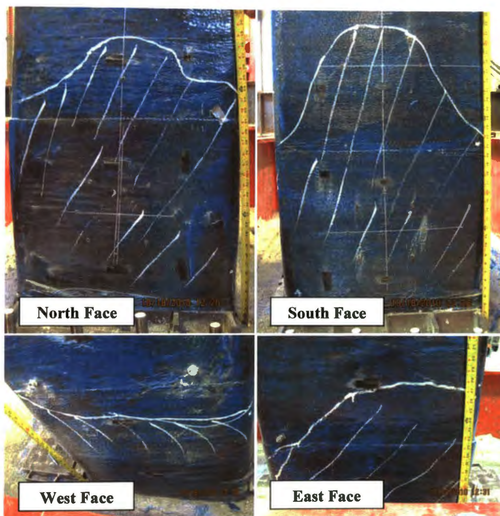
Figure 5.7. Debonded Areas of CFRP on Column #2 After Testing
